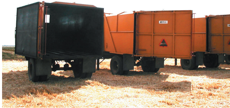
Tubs, or trailers, especially designed for bringing mint from field to still
