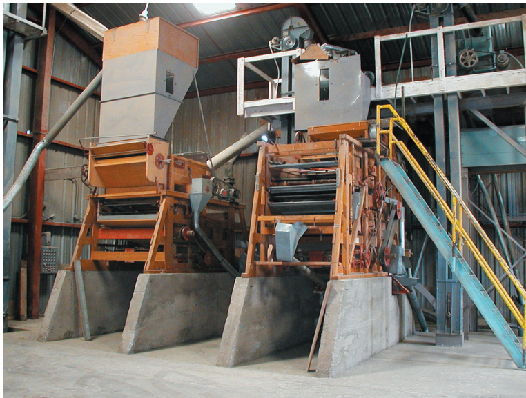
Grass seed cleaning machines (vibrating screens of various degrees of fineness)
