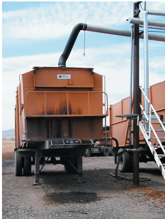
Steam ejected from pipes in floor of tub passes through mint; mint oil passes through pipe at top to still
