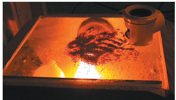
Grass seed being examined for purity-- spread on glass-topped light box Photo by Eugene Smith
